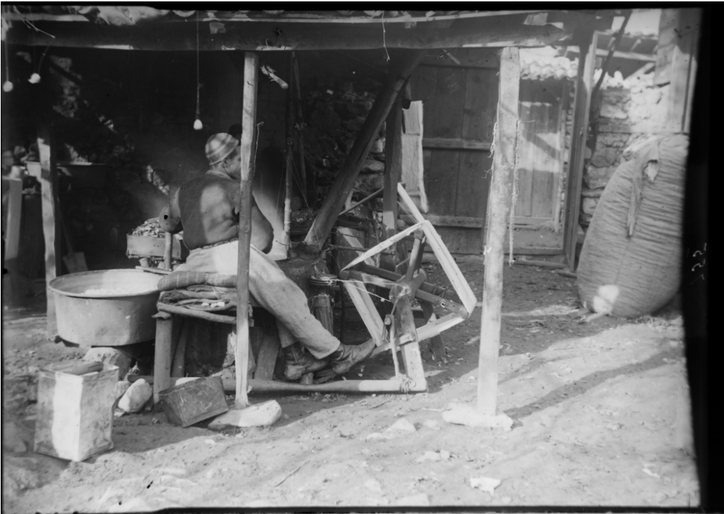
Reeling a thread from the cocoons of Bagdad White species on a local loom Source: Silk Museum Photo Collection , IIIF Manifesto
